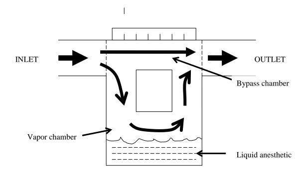
Figure 2. Schematic diagram of a precision vaporizer
